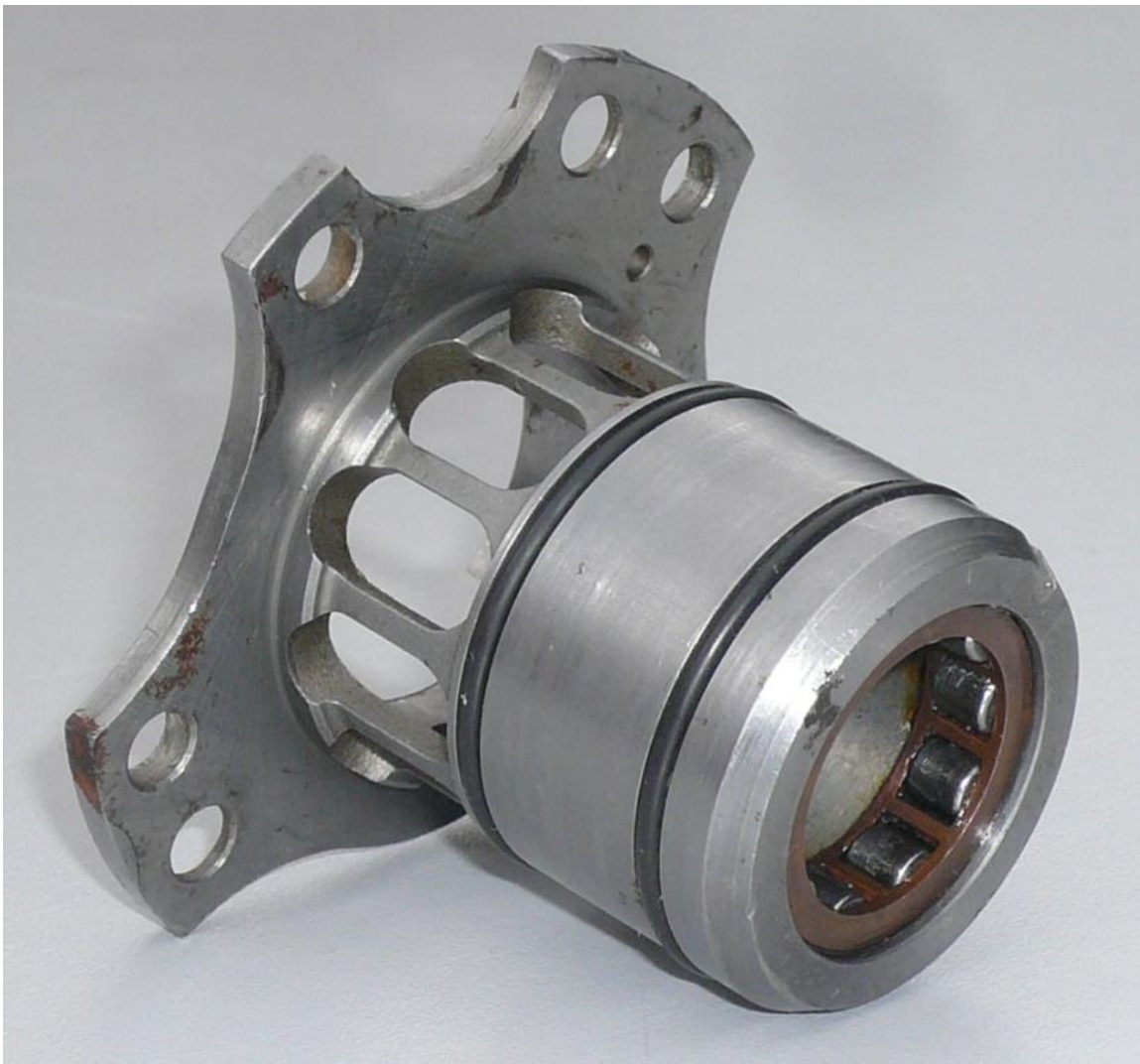
Bearing carrier mounted as oil-damped sprung piston
