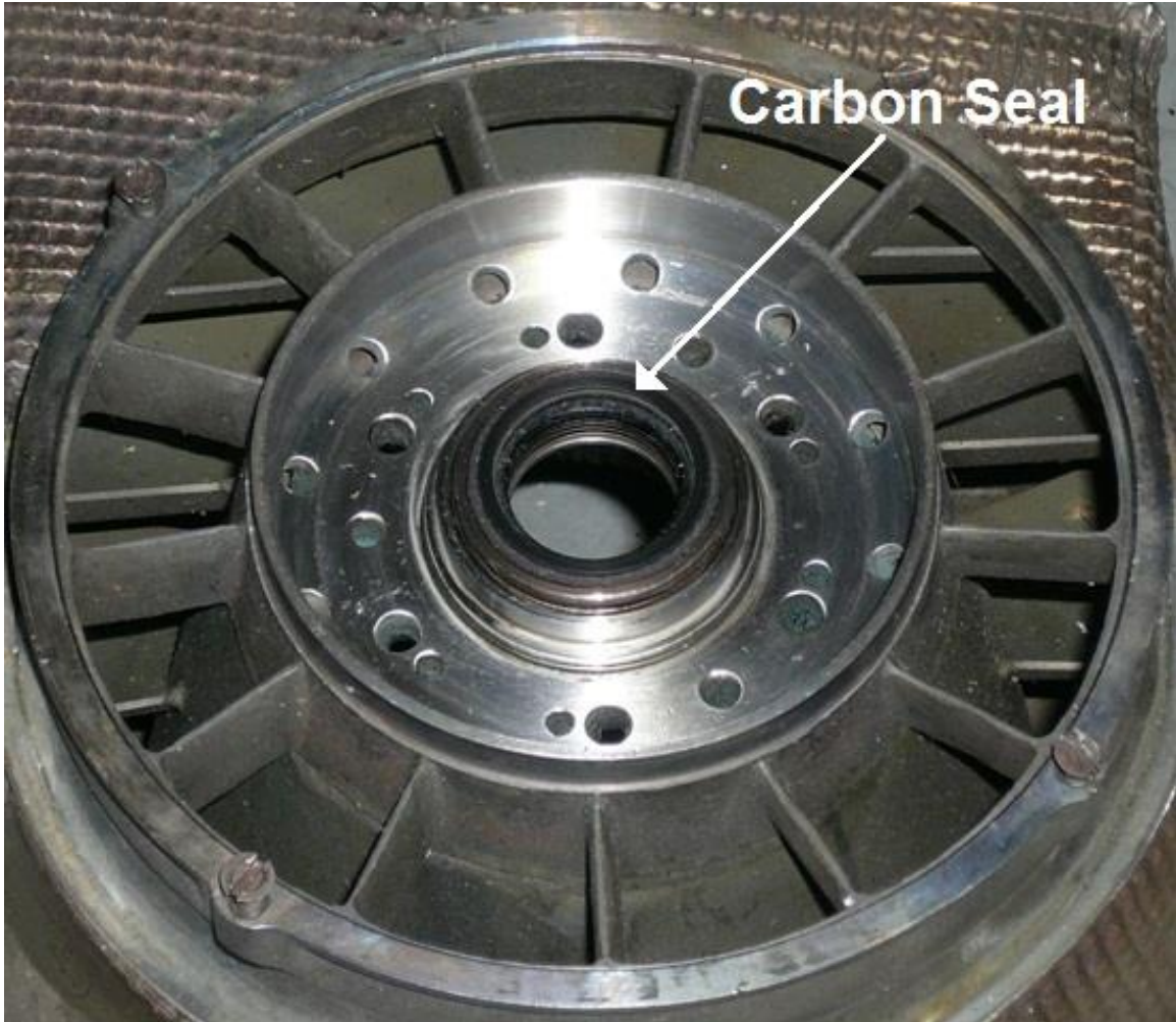
Carbon shaft seal (turbine wheel removed-Plessey Solent MK101)
