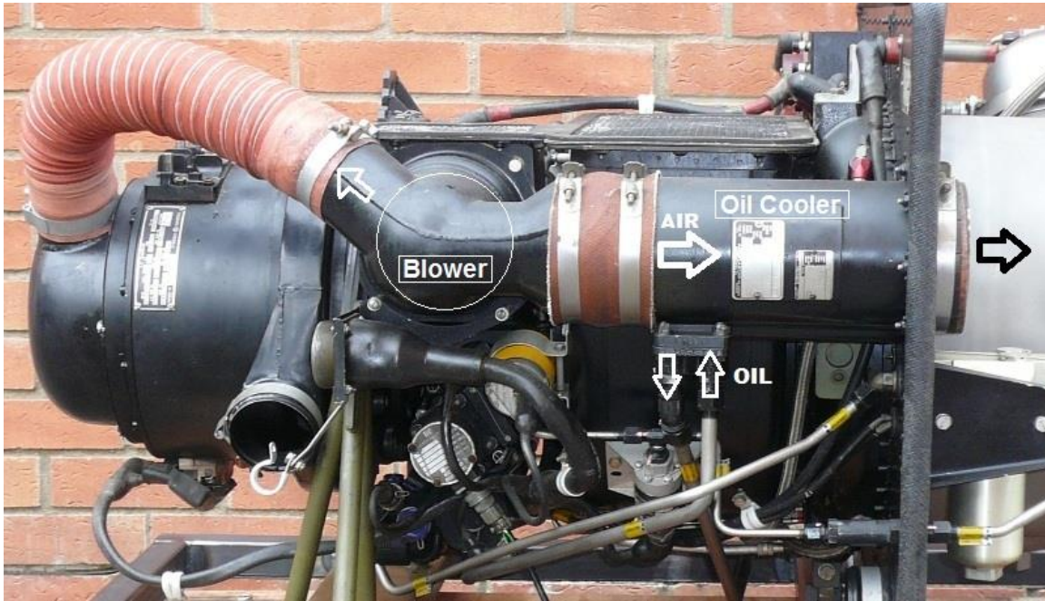
Oil cooler radiator fed from engine-driven blower
